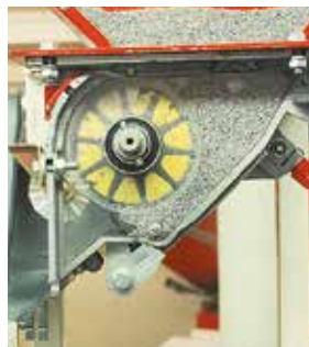
Setting for fine seeds, with rotary brush
