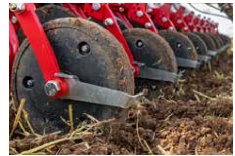
On slightly sticky soils an optional scraper is recommended for the press wheel.
