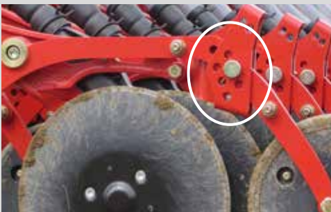
The press wheel can be set in several positions to ensure perfect seed placement coulters by coulters.
