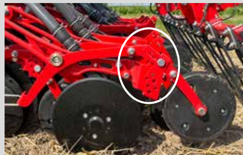
Lifted press wheel setting recommended in wet and sticky conditions.
