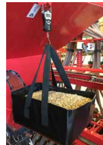
A calibration bag and set of digital scales are supplied as standard. The calibration tests are carried out electronically rather than manually.
