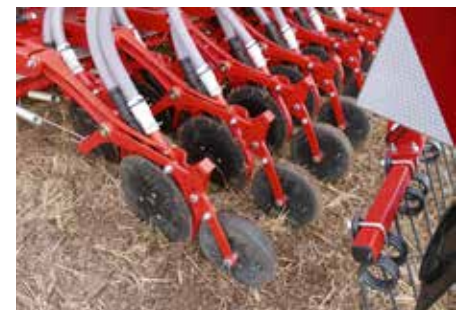
CX-II coulters double entry for application of two products (e.g. fertilizer and seeds) in one pass.
