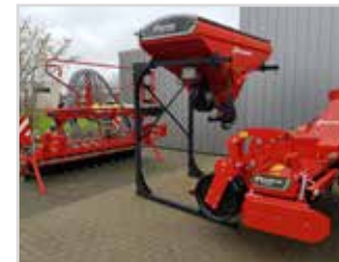
Flexible use of the power harrow whether with seed hopper or in solo operation depending on soil conditions.
