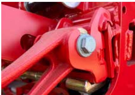
Clamped brackets of the CX-II coulters to be flexible in row spacing.
