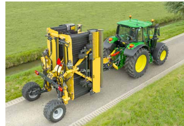
The Kverneland ROC RS 730 can be folded into a width of only 2.5 meters for road transport.
