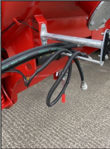
Hose and Cable Storage
