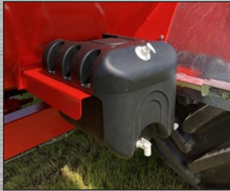
Hand Wash Tank
