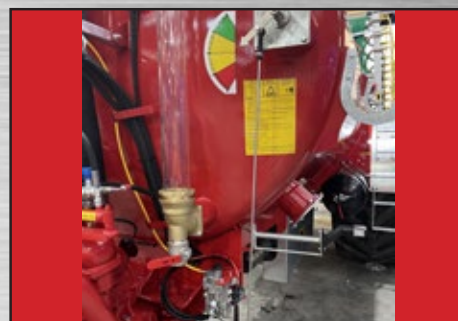
Float Type Level Indicator c/w Load Sensing for Brakes
