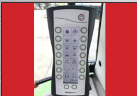
LCD Controller for Electro - Hydraulic Control
