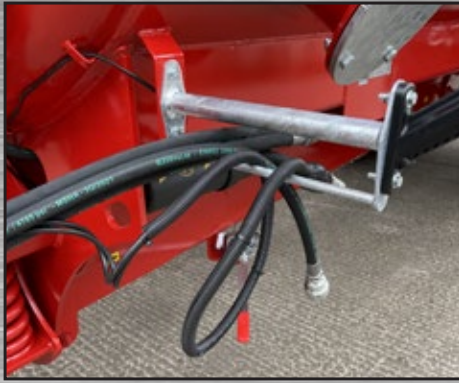
Hose & Cable Storage
