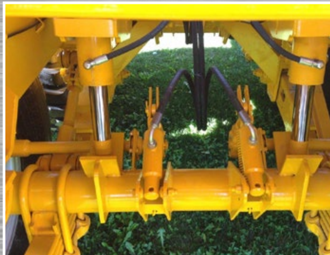
Automatic Weight Transfer System (Manual version Standard on 20 Tonne)
