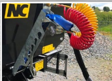
Air & Hydraulic Brakes or Air Only Brakes
