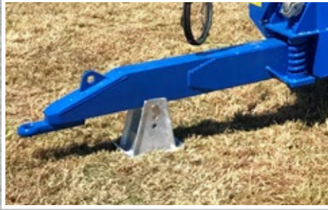
Sprung Drawbar Complete with Galvanised Parking Stand
