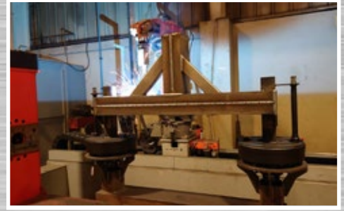
Robot Welded Rocking Bogie
